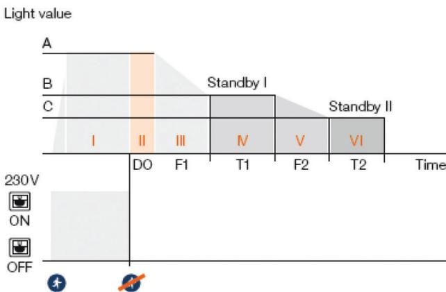
Three dimming ranges (1...100%), free parameterization of time (I...VI) using DALI magic.
