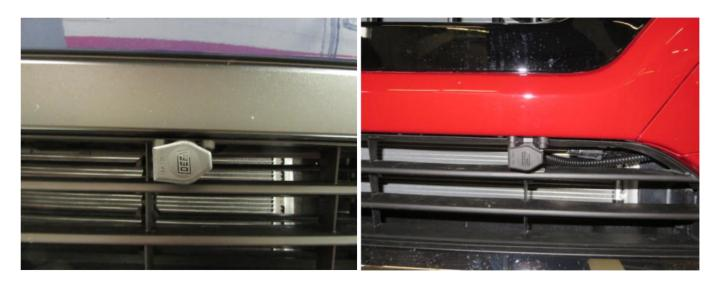
If installing the cable through the grill mesh, Install the Inlet cable through a hole in the grill and secure the MiniPlug socket to the grill using the assembly ring **(A)**, the 55mm disc **(I)** and the locking collar **(F)** to secure the MiniPlug to the grill in the location indicated in the pictures below and as shown on pages 6 and 7.
