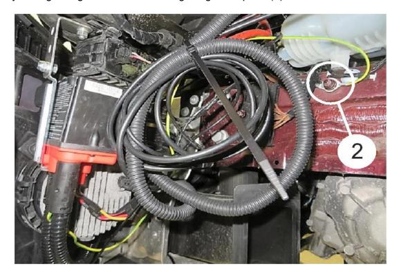
Install the battery charging wire harness between the charger and the battery and secure it along the original wire harnesses using the provided zip ties. Connect the positive lead of the wire harness to the positive battery post or clamp and secure the fuse holder with a plastic cable tie. The red wire can also be connected to the positive power connection of the underhood fuse panel. Attach the black ground lead to an original ground point on the chassis.
