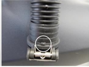
**NOTE:** Remove only one of the plastic drains (the one that will be at the bottom) as pictured below and as shown in detail picture number 5 on page 7 of these instructions. Failure to do so may result in corrosion inside the socket.
