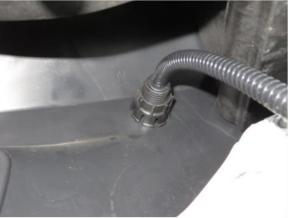
If using the mounting bracket in the grill, use the mounting bracket **(G)** to secure the MiniPlug to the upper part of the grill opening. Use the small screws **(H)** to lock the bracket into position on the MiniPlug housing. Use the self-tapping screws **(D)** to install the assembled MiniPlug on the front bumper as shown in the picture below. If needed, the bracket shim **(C)** can be used between the bracket and the bumper cover mounting area to gain extra MiniPlug flap opening clearance.
