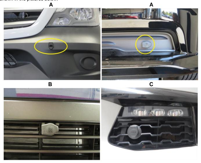
If method A is preferred, drill a 24mm (15/16ths inch) hole in the desired location and make a 3mm groove at either the 9, 12 or 3 o'clock position depending on if the flap will be opened vertically or horizontally.
