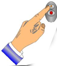
After the fourth figure has been entered, the immobilizer turns itself off after a couple of seconds, as long as the correct code has been entered! If you enter the wrong code (e.g. enter the wrong number for the second figure), you must still complete the other figures, or wait for 20 seconds to try again from point 1.
