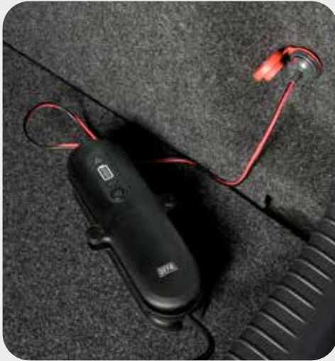
12V charging socket can be used to recharge your battery or as a power supply when you need it.
