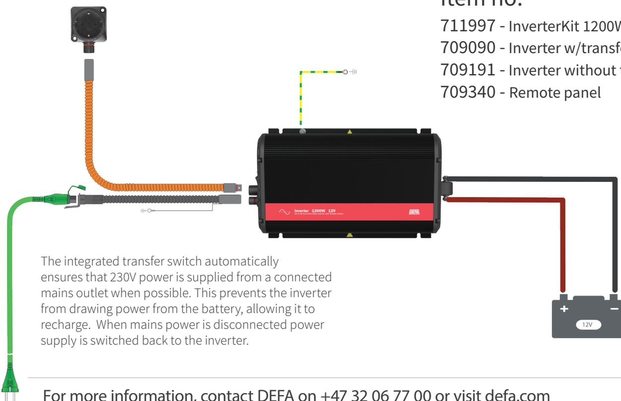
The integrated transfer switch automatically ensures that 230V power is supplied from a connected mains outlet when possible. This prevents the inverter from drawing power from the battery, allowing it to recharge. When mains power is disconnected power supply is switched back to the inverter.
