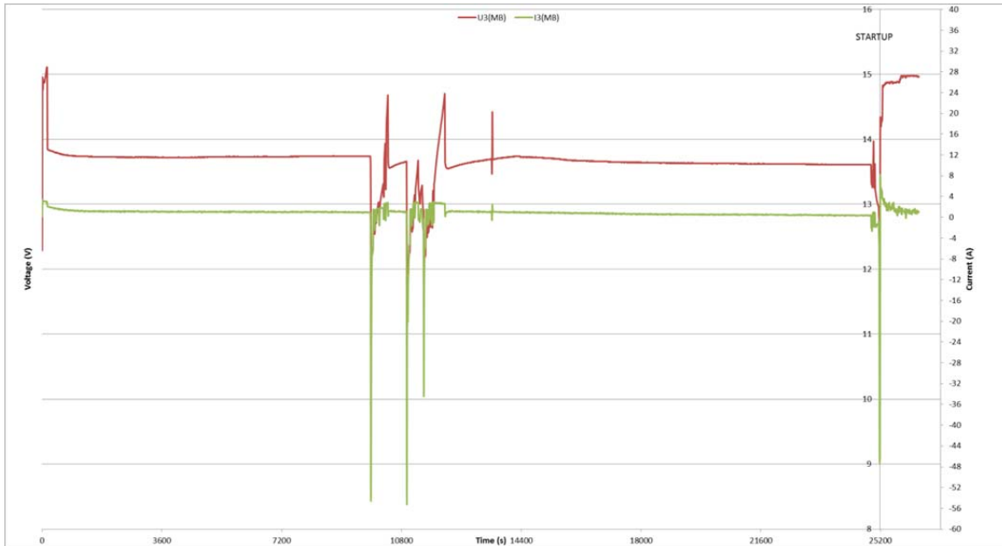
Figure 4. The voltage/current graph of test D5 during the pre-charging and preheating period.
