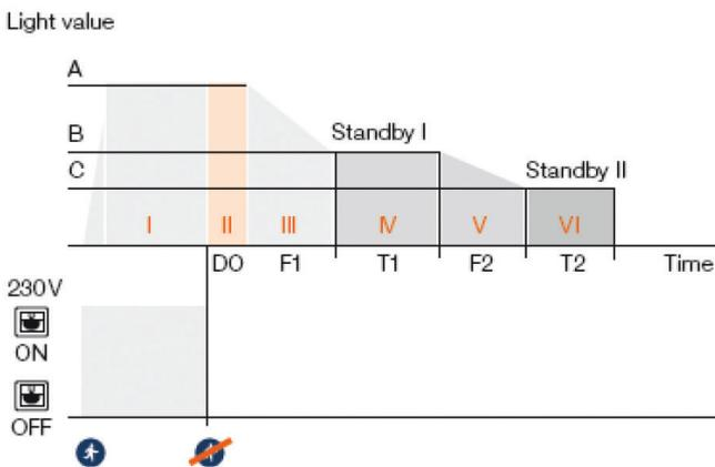
Three dimming ranges (1...100%), free parameterization of time (I...VI) using DALI magic.
