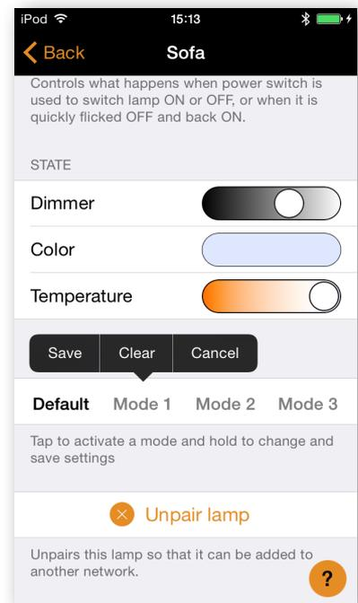
*Tip: Create a standard step dimmer by storing Mode 1 = 75%, Mode 2 = 50% and Mode 3 = 25%.*
