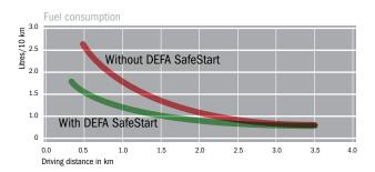
Starting of a preheated engine reduces the fuel consumption with 50% the first 4  $\mbox{km}$
